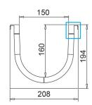
Watertight: to ensure the watertight of the channels, it is advisable to use a bituminous sealing adhesive. As a complete and long lasting guarantee of the absence of leakages through the joints of the channels, it is possible to heat-weld the joints.
