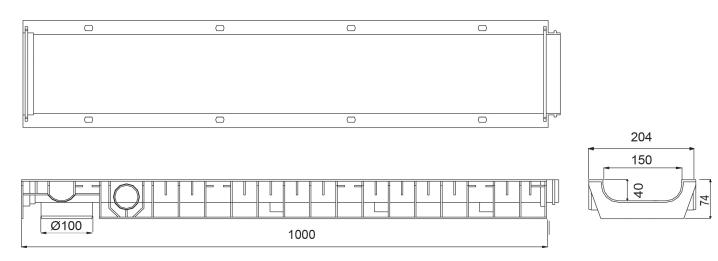
Watertight: to ensure the watertight of the channels, it is advisable to use a bituminous sealing adhesive. As a complete and long lasting guarantee of the absence of leakages through the joints of the channels, it is possible to heat-weld the joints.
