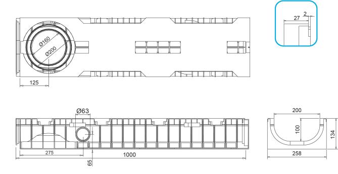
Watertight: to ensure the watertight of the channels, it is advisable to use a bituminous sealing adhesive. As a complete and long lasting guarantee of the absence of leakages through the joints of the channels, it is possible to heat-weld the joints.
