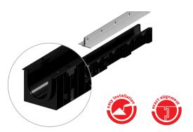
BrickSlot H80 "T" section is designed for **EASY** channel made of HD-PE with no rails. The absence of the rail ensures that the grating completely covers the channel. BrickSlot H80 "T" section can be installed on Easy 100 in all its internal heights: 55, 80, 100 and 160mm.
