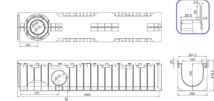
Watertight: to ensure the watertight of the channels, it is advisable to use a bituminous sealing adhesive. As a complete and long lasting guarantee of the absence of leakages through the joints of the channels, it is possible to heat-weld the joints.
