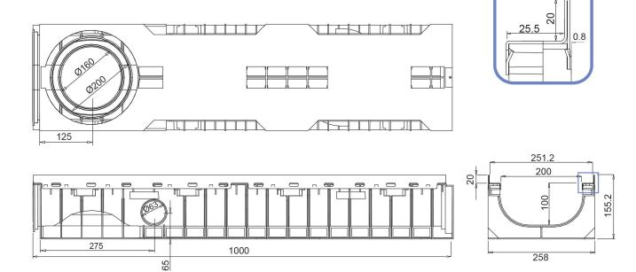
Watertight: to ensure the watertight of the channels, it is advisable to use a bituminous sealing adhesive. As a complete and long lasting guarantee of the absence of leakages through the joints of the channels, it is possible to heat-weld the joints.
