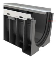
The steel rail is 20 mm high and 2.5 mm thick in the area exposed to vehicle transit. It holds the gratings and helps in an easy installation of the channel system.
