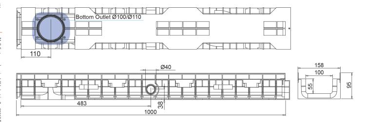
Watertight: to ensure the watertight of the channels, it is advisable to use a bituminous sealing adhesive. As a complete and long lasting guarantee of the absence of leakages through the joints of the channels, it is possible to heat-weld the joints.
