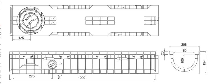
Watertight: to ensure the watertight of the channels, it is advisable to use a bituminous sealing adhesive. As a complete and long lasting guarantee of the absence of leakages through the joints of the channels, it is possible to heat-weld the joints.
