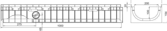
Watertight: to ensure the watertight of the channels, it is advisable to use a bituminous sealing adhesive. As a complete and long lasting guarantee of the absence of leakages through the joints of the channels, it is possible to heat-weld the joints.
