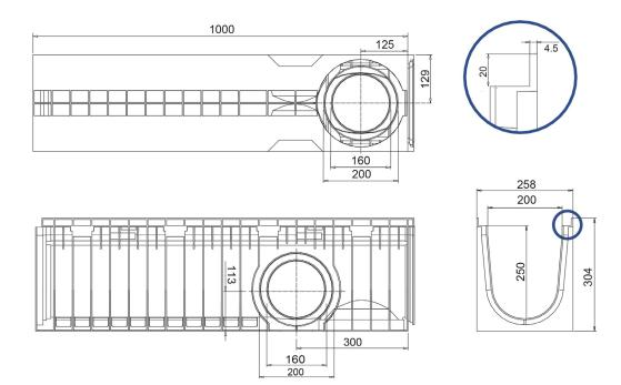
Watertight: to ensure the watertight of the channels, it is advisable to use a bituminous sealing adhesive. As a complete and long lasting guarantee of the absence of leakages through the joints of the channels, it is possible to heat-weld the joints.
