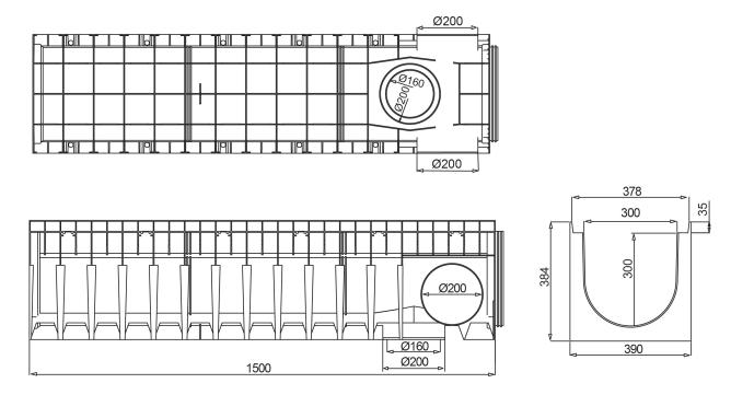
Watertight: to ensure the watertight of the channels, it is advisable to use a bituminous sealing adhesive. As a complete and long lasting guarantee of the absence of leakages through the joints of the channels, it is possible to heat-weld the joints.
