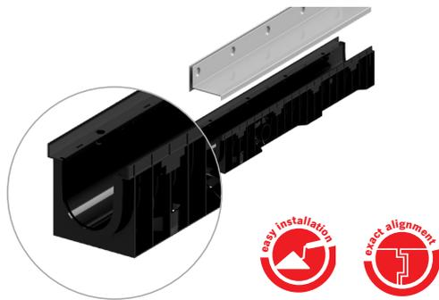
BrickSlot H80 “L” section is designed for **VIP** channel made of HD-PE with an inbuilt rail that ensures protection on the gratings. BrickSlot H80 “L” section can be installed on Vip in all its internal heights: 55, 80, 100 and 160mm.
