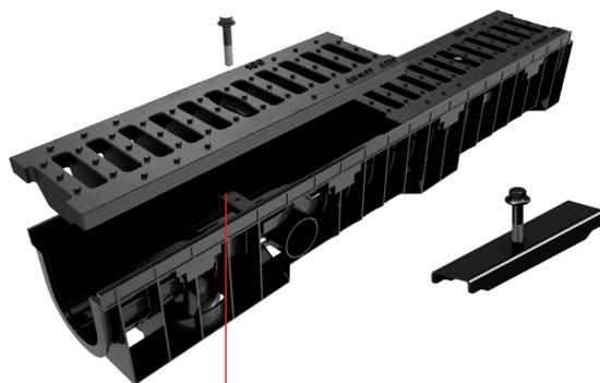
To fix the gratings on the Mufledrain VIP channels with internal width 100, 150 and 200 mm, you will need one bar and bolt every half meter of channel.
