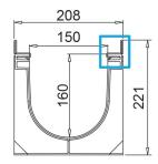
Watertight: to ensure the watertight of the channels, it is advisable to use a bituminous sealing adhesive. As a complete and long lasting guarantee of the absence of leakages through the joints of the channels, it is possible to heat-weld the joints.
