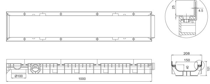
Watertight: to ensure the watertight of the channels, it is advisable to use a bituminous sealing adhesive. As a complete and long lasting guarantee of the absence of leakages through the joints of the channels, it is possible to heat-weld the joints.
