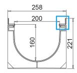
Watertight: to ensure the watertight of the channels, it is advisable to use a bituminous sealing adhesive. As a complete and long lasting guarantee of the absence of leakages through the joints of the channels, it is possible to heat-weld the joints.
