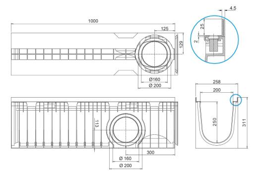
Watertight: to ensure the watertight of the channels, it is advisable to use a bituminous sealing adhesive. As a complete and long lasting guarantee of the absence of leakages through the joints of the channels, it is possible to heat-weld the joints.
