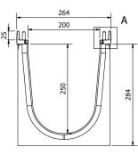
Watertight: to ensure the watertight of the channels, it is advisable to use a bituminous sealing adhesive. As a complete and long lasting guarantee of the absence of leakages through the joints of the channels, it is possible to heat-weld the joints.
