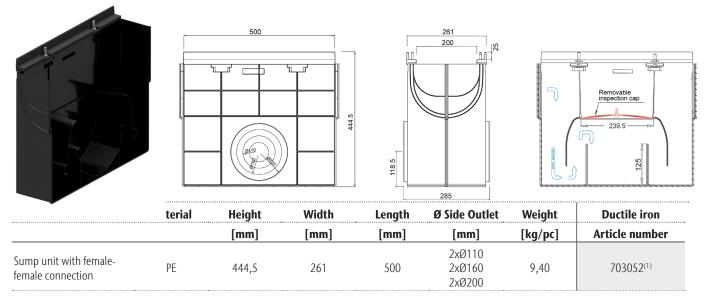
$^{\scriptscriptstyle (1)}\text{It}$  is not designed for connection to H250 channels
